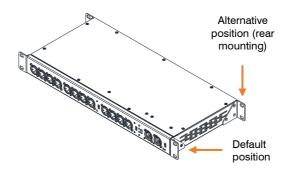
① Only use the M3x5mm countersunk screws provided with the unit.
